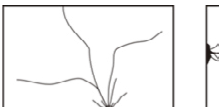
Fig. 31 GLASS DEFECTS (impact on the edge)
