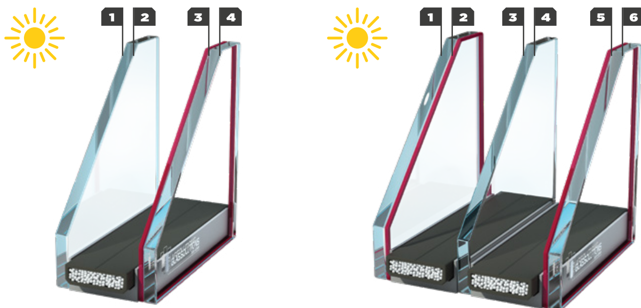
Fig. 3 Numbering of items in a single-glazed and double glazed unit Source: own study
